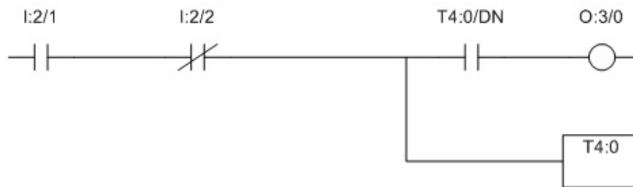
Figure 4.14: Ladder Logic: Elimination of Race Condition
