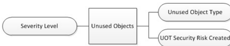
Figure 4.9: Ladder Logic Vulnerability Taxonomy: Unused Objects Installed
