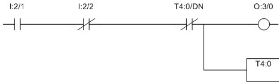
Figure 4.11: Race Condition: Ladder Logic Incorrect
